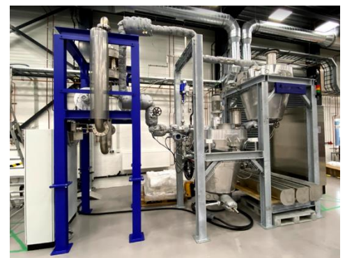
Figure 1 overview of the hot air (left) and molten salt (right) test facilities in the Carnot Lab.
