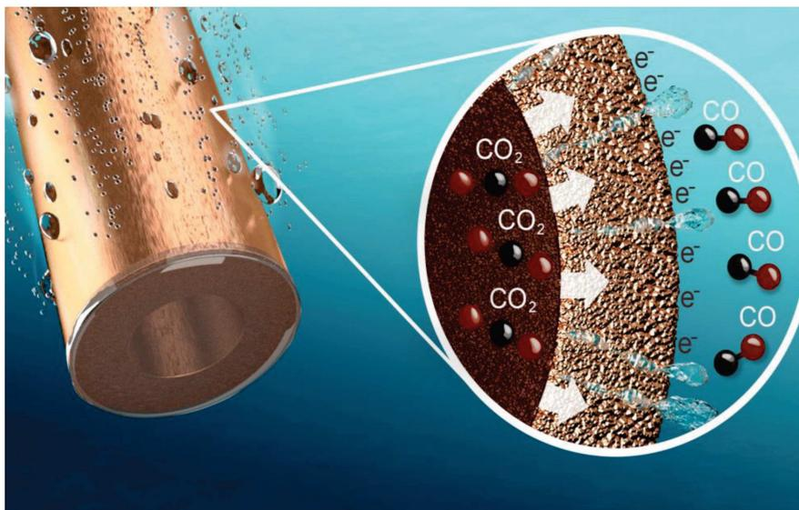
Copper hollow fiber electrode for carbon dioxide conversion. From DOI: 10.1038/ncomms10748.
