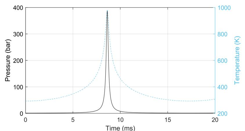
Figure showing the modelled temperature and pressure during a compression.
