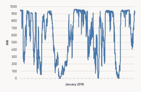
Power supply to a 1 GW green hydrogen plant based on a typical North Sea wind pattern. The graph is based on 2018 data of a 950MW North Sea wind park, adjusted to gigawatt scale.
