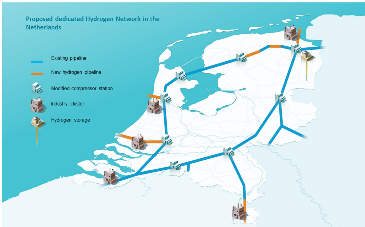
Figure 6: Visualisation of the Gasunie hydrogen backbone. [source: Gasunie]
