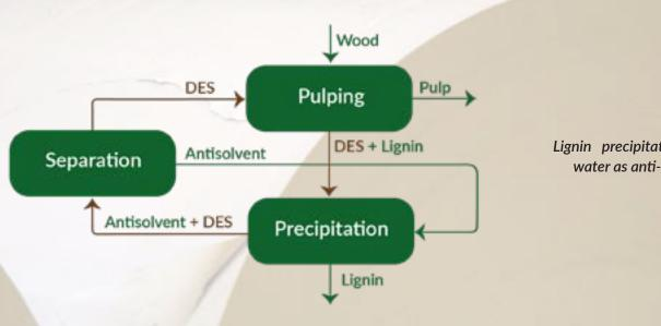
Lignin precipitation using water as anti-solvent
