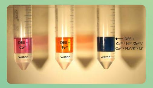
A variety of hydrophobic DESs were tested on the dissolution of specific contaminants. Hydrophobic DESs appear able to dissolve volatile fatty acids, 6 metal ions, 7 and some ink and sticky contaminants. Although the mineral oil content was halved, deinking trials did not lead to higher brightness.
