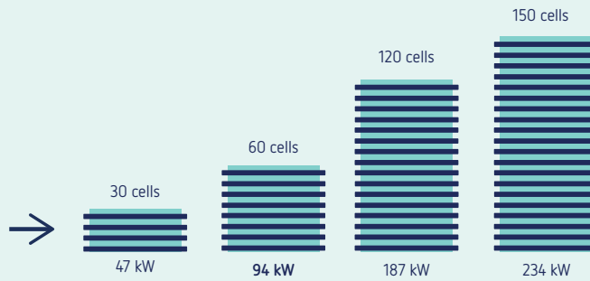
Figure 14. Scaled-Up SOE Stacks. Two upscaled options are emphasized: 94 kW stack of 120 cells of 400 cm 2 at 1.5 A/cm 2 thus 156 V @ 600 A and 94 kW stack of 60 cells of 800 cm 2 at 1.5 A/cm 2 thus 78 V @ 1,200 A
