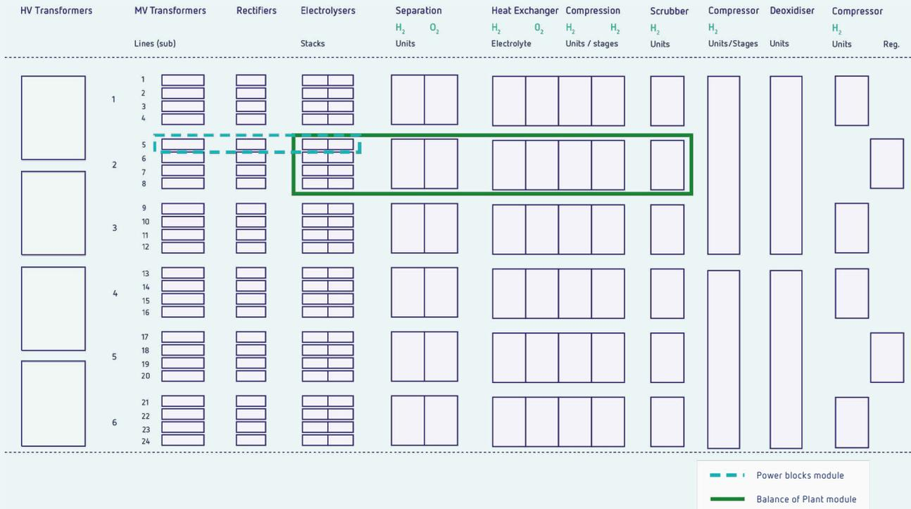
Figure 4: General layout of a modular large-scale water electrolysis plant with multiple stacks and separators (Alkaline)
