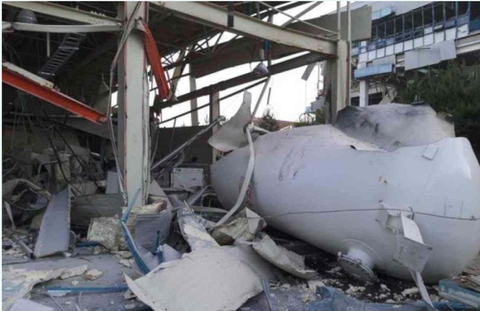
Figure 11: Hydrogen tank explosion at a pilot plant facility, South Korea, 2019
