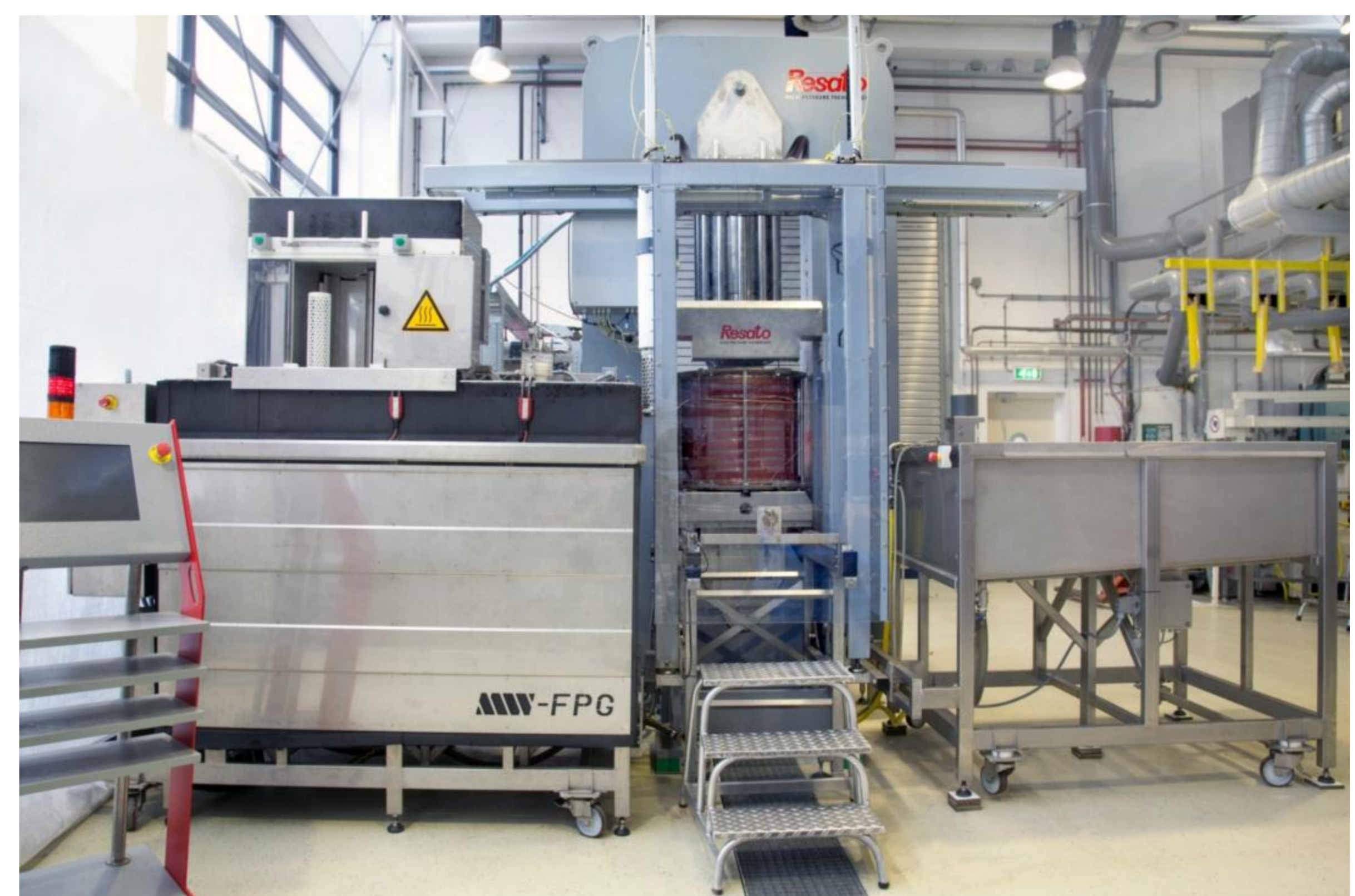
Pilot unit for high pressure high temperature processing
